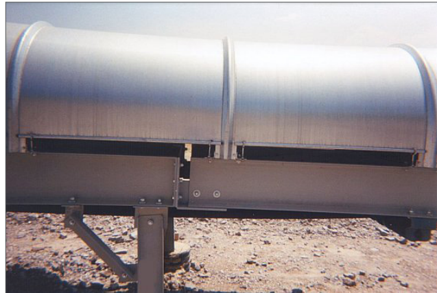
Half-moon covers (similar to above) would be utilized over most sections of the Central Conveyor to inhibit rain, wind and fugitive dust.
